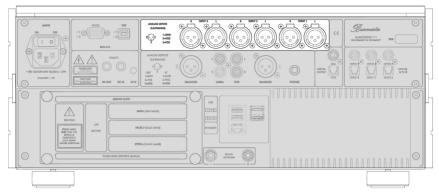
► Connect analog signal sources to INPUT 1/2/3 using balanced LF cables. Unbalanced cables can be connected using the XLR-RCA adapters supplied with the device.
