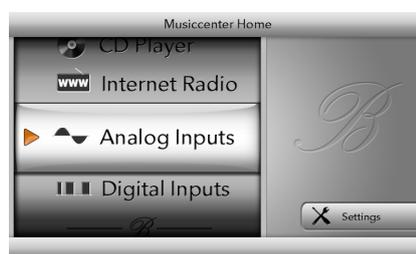
3. Scroll through the inputs by turning the left rotary dial and push it to make your input selection.
