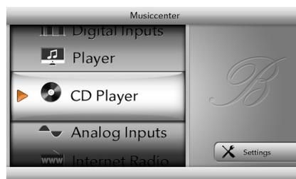
2. Select **Analog Inputs** or **Digital Inputs** by turning the left rotary dial and push the dial in to select the respective menu window.
