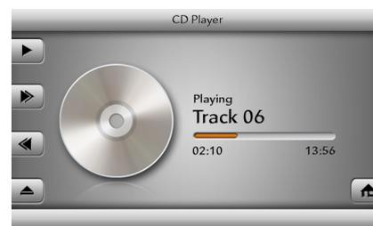
2. To operate the CD player please use the left row of tabs on the screen or the relevant buttons on the remote control.
